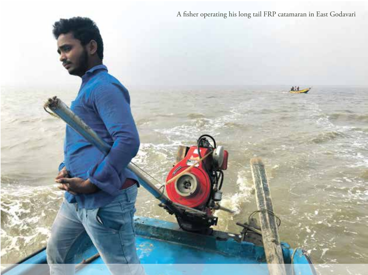
FRP catamaran with a modified rear to optionally attach an outboard motor
