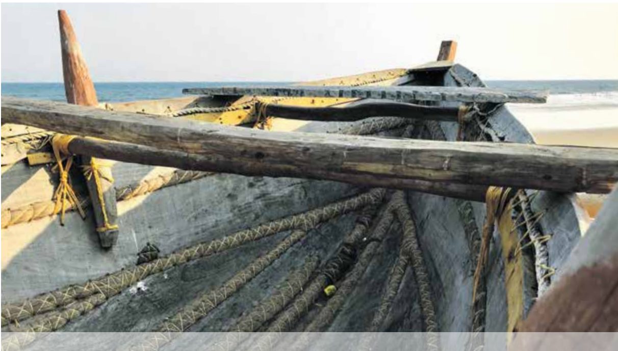
Interior of the big stitched wooden boat which is used for shore seine fishing. In the image here, the stitching between planks is visible. These are lined with a coastal grass that is water resistant and supports the buoyancy of the craft. There are currently only a handful of boat makers who have the knowledge and know-how to build this type of craft.
