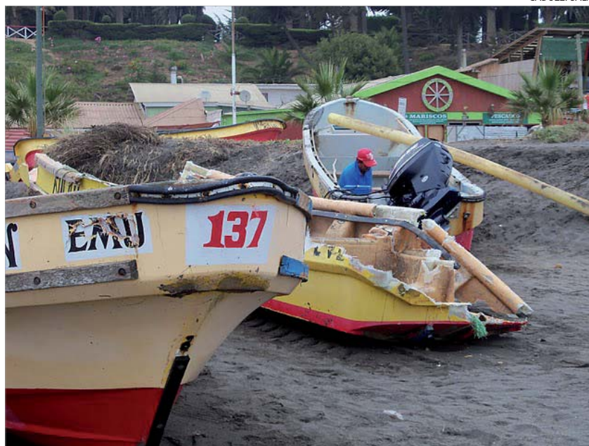
Pichilemu beach, O'Higgins Region, Chile. Damaged 7-9-m fiberglass fishing vessels used to catch common hake and crabs
