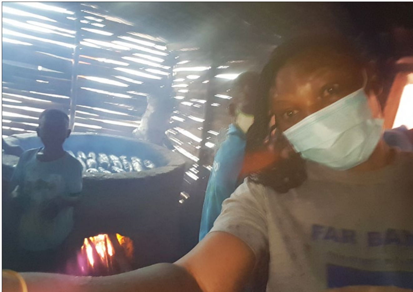
Fishmongers using the chorkor smoker, which is quite popular because of its low cost of construction, but which poses a health risk to fish processors as they have to endure its higher rate of combustion
