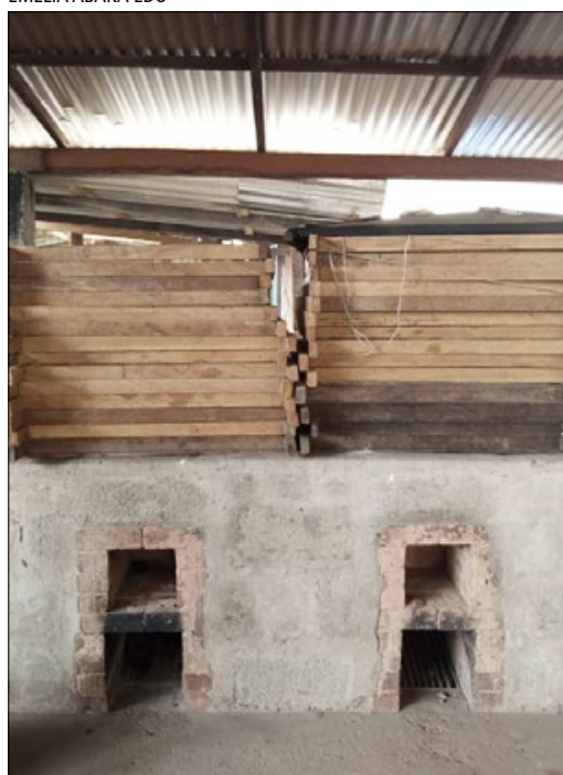
The ahotor oven is energy efficient and helps women fish processors reduce the quantity of firewood in smoking fish. It also improves quality of smoked fish
